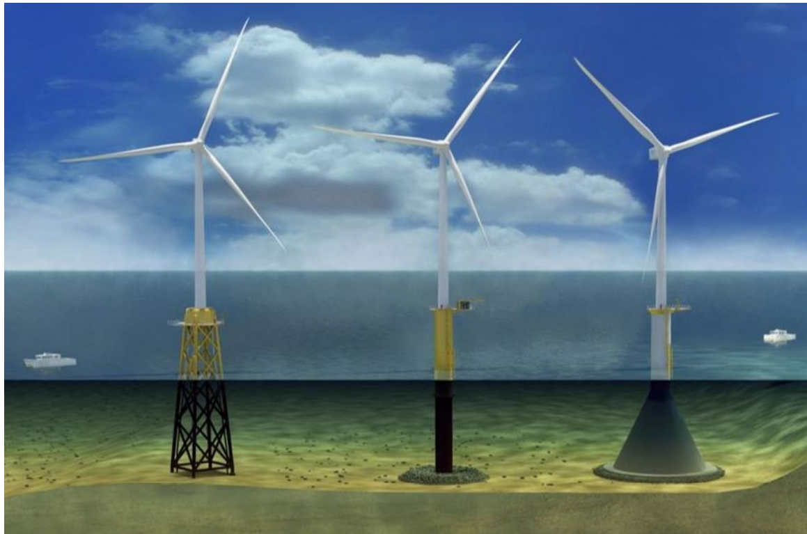
Figure 1: Foundation Concepts Including Jacket, Monopiles, and Gravity-based
